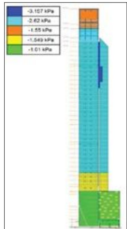
Fig. 13 : Wind Pressure Thro CFD
