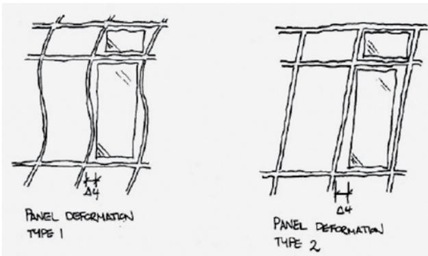
Fig. 2 : Panel Mode of Movement Due to Sway
